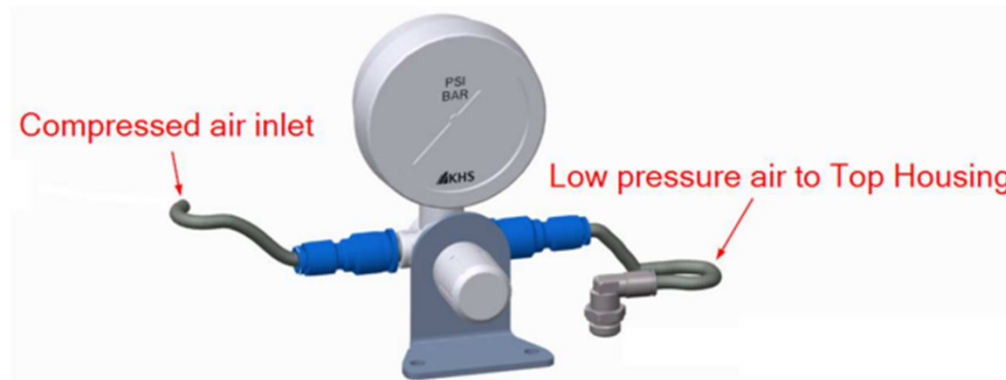
Figure 5-41: Seamer internal positive pressure control
