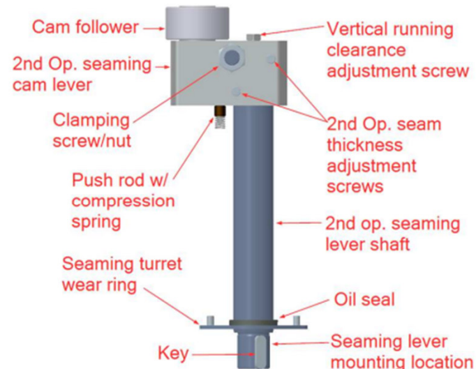
Figure 5-25: 2 nd Op seaming lever shaft
